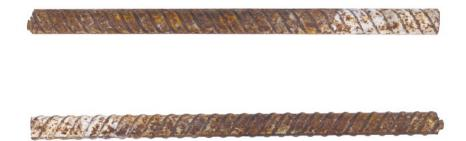
The effects of galvanic corrosion on reinforcing steel.
